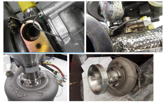
Examples of incorrect sealing wiring
